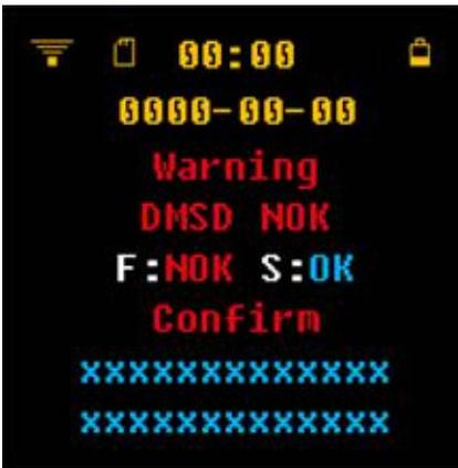
The warning message "DMSD NOK" indicates the type of error (force or stroke) that has occurred.
