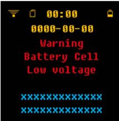
The warning message "Battery Cell Low Voltage" indicates that the battery cell on the power electronics is empty.
