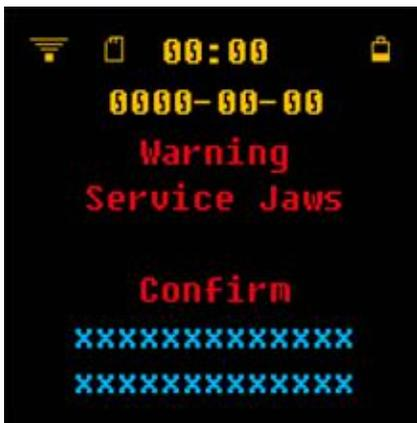
The warning message “Service Jaws” indicates that the clamping jaws need to be serviced or replaced.
