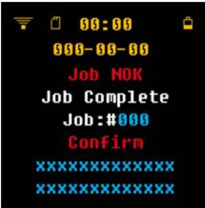
This message is displayed when a job has been completed, i.e. the required number of rivets have been set correctly.
