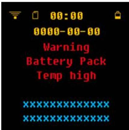
The warning message “Battery Pack Temp High” indicates that the battery is being overloaded.
