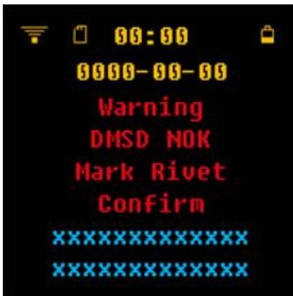
The warning message “Mark Rivet” prompts you to mark the rivet and then to continue riveting in order to finish the job.
