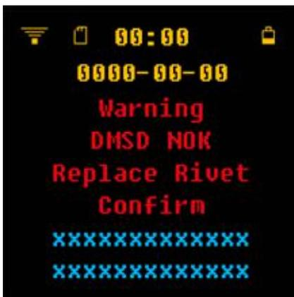
The warning message “Replace Rivet” prompts you to remove the rivet, e.g. by drilling out the faulty rivet, and then to continue riveting in order to finish the job.
