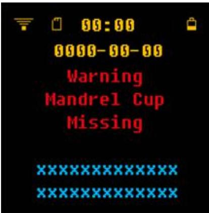
The warning message "Mandrel Cup Missing" indicates that the stud collector is missing or has not been correctly or completely screwed on.
