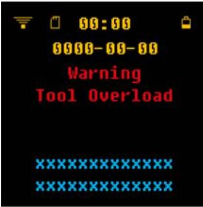
The warning message "Tool Overload" indicates that the RivSmart is being overloaded.
