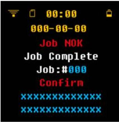
If the DMSD Lite process monitoring system is active in addition to the job, a job error message is also displayed at each DMSD Lite error message.
