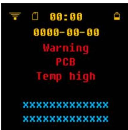
The warning message “PCB Temp High” indicates that the RivSmart is being overloaded.
