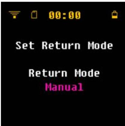
In the “Return Mode” screen you can set whether the riveter moves back to the front starting position after setting the rivet by releasing the trigger or automatically after the shearing of the rivet mandrel.
