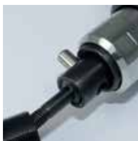
Quick change system for the mandrel.
