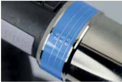
Exact adjustment of the setting stroke via scale on the adjustment cap.
