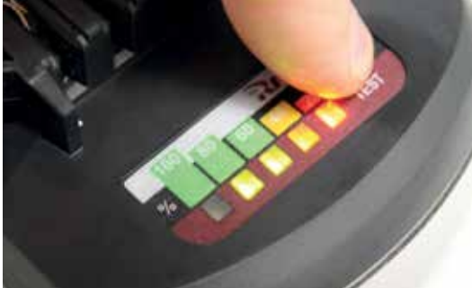
Optical capacity indicator on each Rivdom battery
