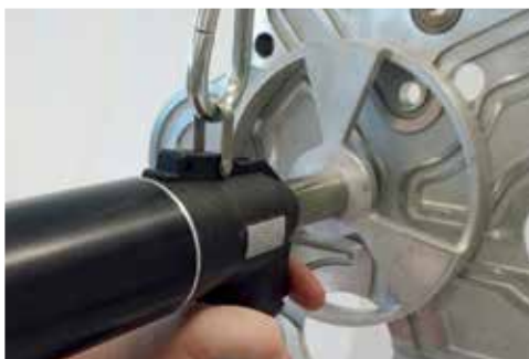
Special accessory angular adapter for keeping the need rectangularity to the component.
